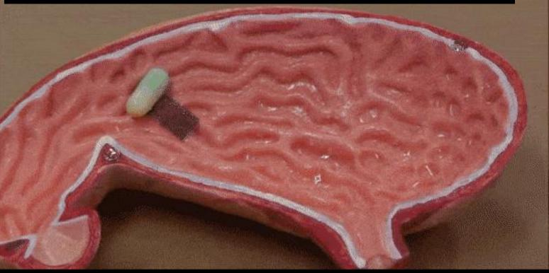
"The robot is fabricated with a silicon material called polydimethylsiloxane (PDMS) embedded with magnetic particles, which allows it to be remotely controlled by applying electromagnetic force. Increasing the frequency increases the speed"
